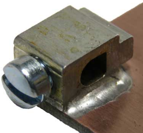
Figure 12. Shows a strong fillet on the counterclockwise torque lateral edge line.
